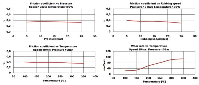
Rubbing speed, temperature and pressure are related. Changing any values will change other. The values shown represent typical conditions, but are not ultimate limits of the material.
